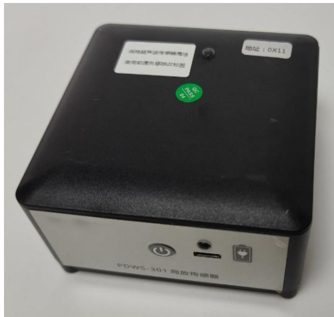
Wireless ultrasonic / transient ground voltage dual-mode sensor
