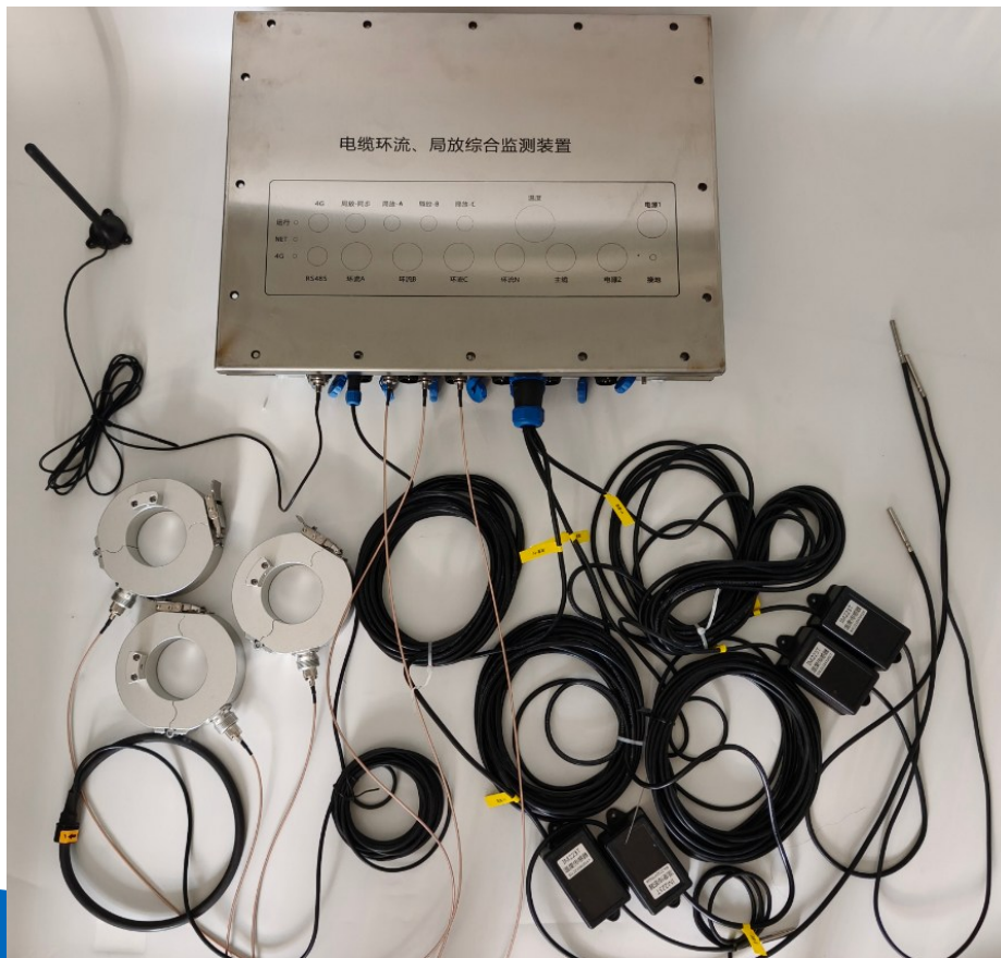
High-Voltage Cable Circulating Current and Partial Discharge Integrated Online Monitoring Device
